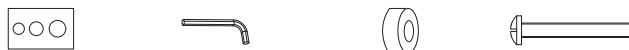
(E) Square Washer (4) (F) Allen Key(1) (G) 5mm Plastic Sleeve(4) (H) M5x40 screws(2)
